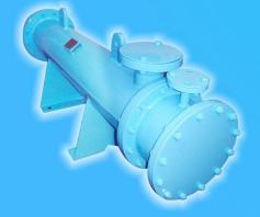
A shell and tube heat exchanger is the most common type of heat exchanger in all Industries. Mostly used in higher-pressure and Higher Temperature applications. This Type of Heat exchangers are having two divisions one is shell and other is Tubes. Here One fluid runs through the tubes, and another fluid flows over the tubes (through the shell) to transfer heat between the two fluids. For this purpose seamless/ERW or Rolled pipes are used for shell. And Seamless tubes are used for Tubes.
